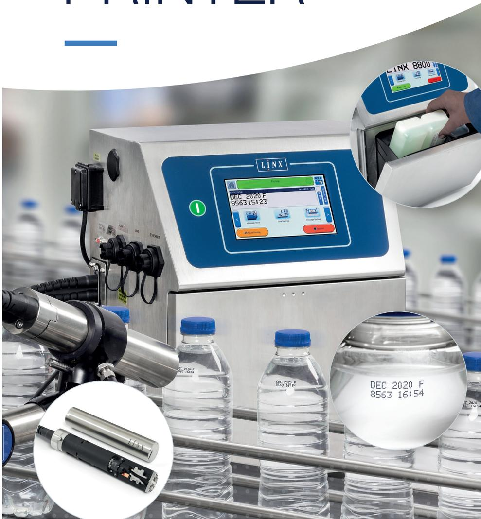
**The Linx 8830 continuous ink jet printer prints up to 3 lines and provides a perfect coding solution for industrial environments.**
