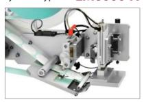
Labeling by extending cylinder arm with label absorbing head. It labels when the product stops moving. It is suitable for jobs requiring accuracy in label position. Air Blow Type
