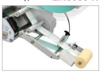
General type of labeling method. It can label on products in motion without stopping. The structure is simple and equipment cost is economical.
