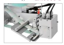
Labeling method is non-contact, air blow type. It can surely label on uneven or bumpy product surface.
